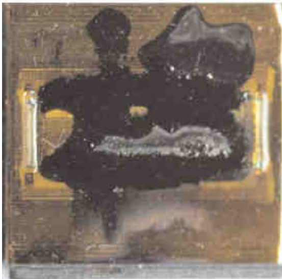
This dirty printhead requires wiping.
